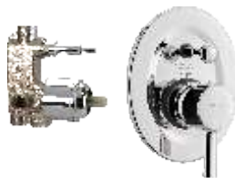
5-way (3 inlets + 2 outlets) single lever concealed diverter system consisting of Exposed part (lever, tip ton knob, wall flange) and Concealed part (cartridge with button assembly, cartridge sleeve) Exposed part F1017711 Concealed Part F4020101
