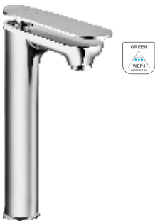
F1018452 Single lever basin mixer with 300 mm (12") extended body and 600 mm braided connection pipe (without pop-up)
