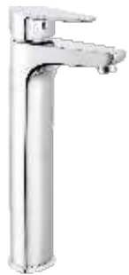
F1013452 Single lever basin mixer with 305 mm (12") extended body and 600 mm braided connection pipe (without pop-up)
