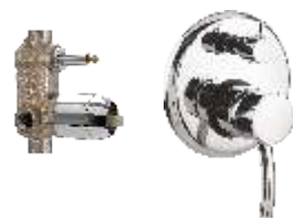
Turn type single lever concealed diverter system consisting of Exposed part (lever, tip ton knob, flange) and Concealed part (40 mm cartridge with button assembly, cartridge sleeve)
